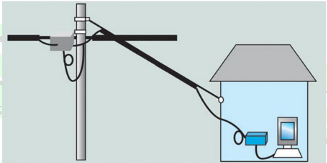
The new design of optical cable sheathed with PE jacket which good for fiber protection in house environment. Furthermore, the cable is located 2 strength member in order to increase it tensile strength. Both FRP or Steel wire would be a choice in this type of cable design. Fiber counts ranged from 1c Singlmode to 12c singlmode which is ideal for the connection between household and the distribution box of the service operators.
